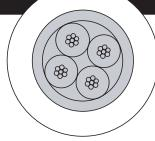
This cable is used for strain gage testing on airframes during flighttesting. It is also used by the automotive industry for crash dummy sensors. This cable uses four conductors insulated with Teflon for reduced size; braided shield for EMI interference and a silicone rubber jacket for flexibility.
